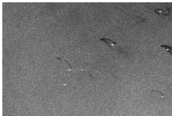
The bright spots in the image are oil platforms off the coast of Norway. The black areas show where water is released by the platforms. This water is slightly oily, though not enough to be in violation of regulations. The radar on Sentinel-1 has the sensitivity to identify these events (Credits: European Space Agency).
